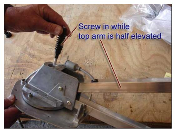
2) Above: Hold the top arm about half way open and screw in the elevating arm.
