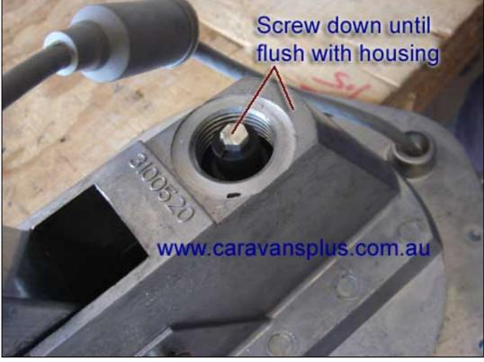
3) Above: Screw down until the top is almost flush with housing.
