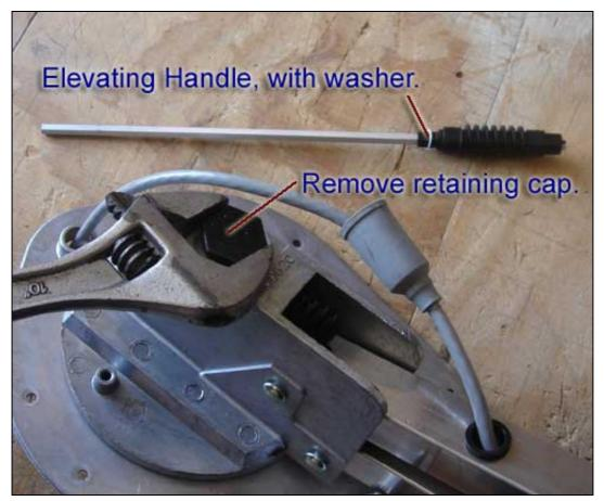
1) Above: Remove the plastic retaining cap.
